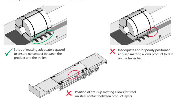
Note: It is important to ensure that the anti-slip matting is visible beneath the product for inspection purposes.
