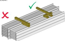
Do not double stack timbers in line, and do not balance timbers on the flanges of beams - create a stable grillage to fill the void.
