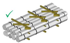
Place packing pieces at an angle to prevent upper timbers sliding off.
