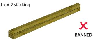
Similar to double stacked dunnage; top timber will still slide off under heavy / emergency braking.
