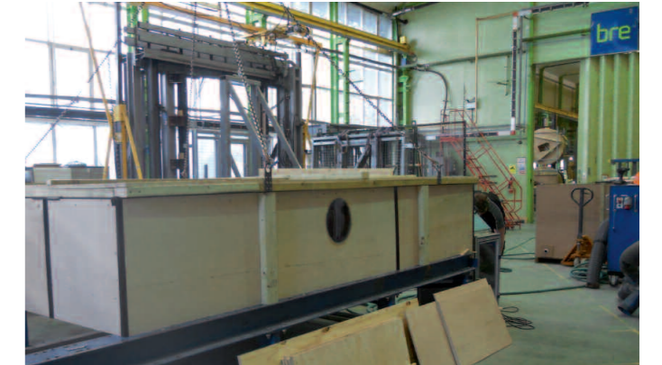
Test apparatus built around specimen and pressurised
