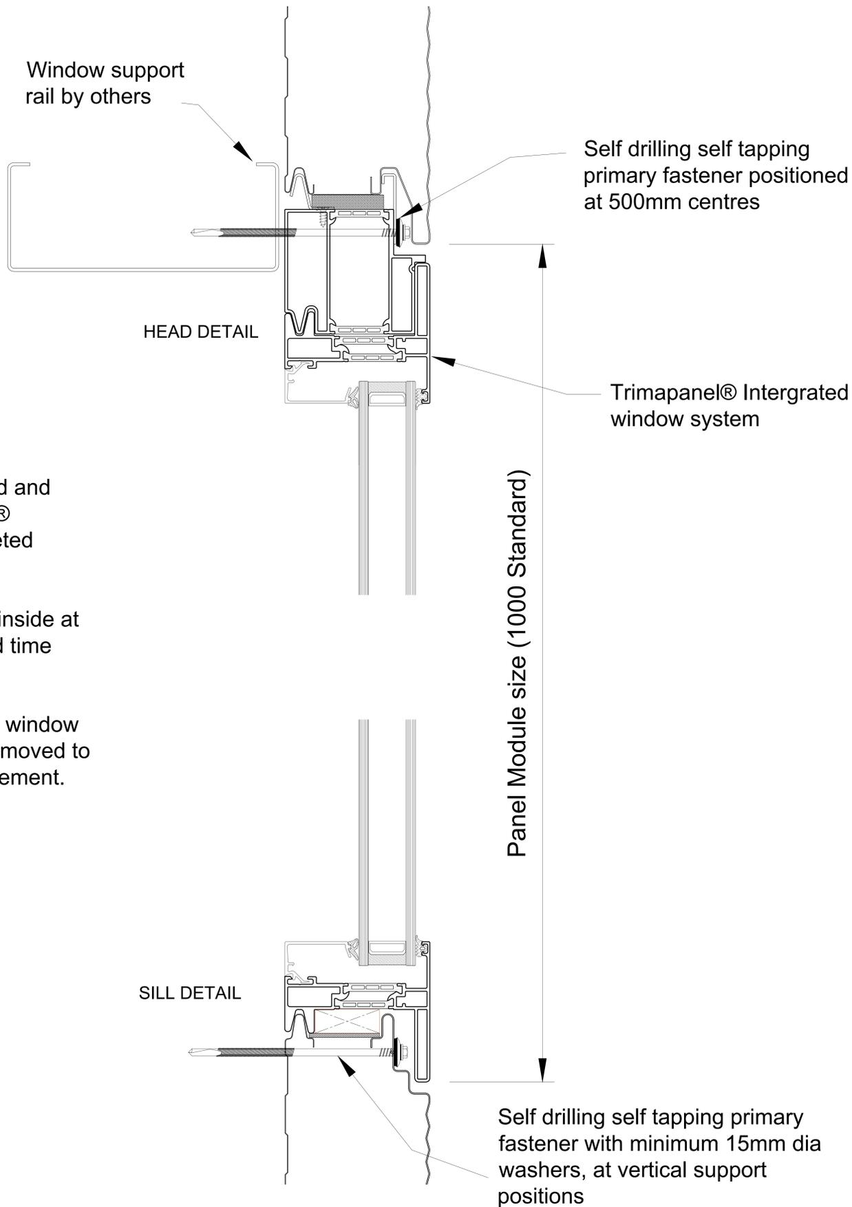
The window frame can be delivered and installed alongside the Trimapanel® allowing the elevation to be completed without delay.
