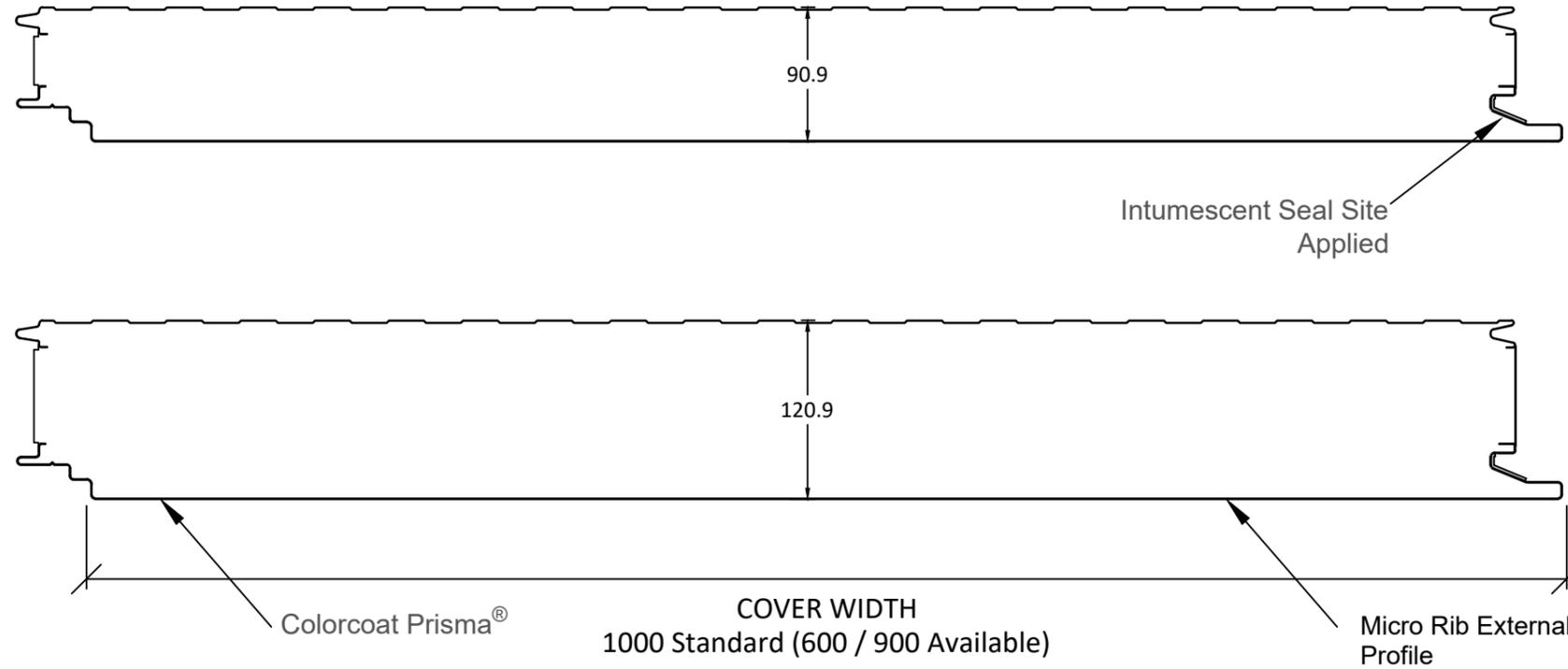
PANEL JOINT & FIXING DETAIL
