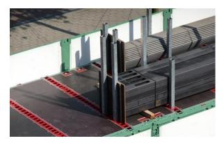
Deck stanchions can be used to produce false headboards, thereby creating a means of blocking whilst maintaining appropriate weight distribution on the vehicle.
