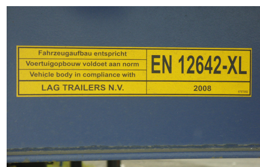
Examples of trailer plaques / signs stating frontwall (headboard) strength and /or compliance with EN 12642 - XL.
