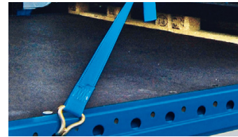
Punched side rave. Rated for 2 tonne webbing straps. Adapter unit available to allow use with higher strength chains.
