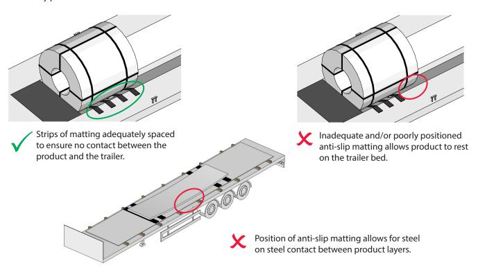
Note: It is important to ensure that the anti-slip matting is visible beneath the product for inspection purposes.
