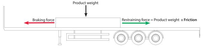
High friction creates more efficient and effective load restraint systems.
