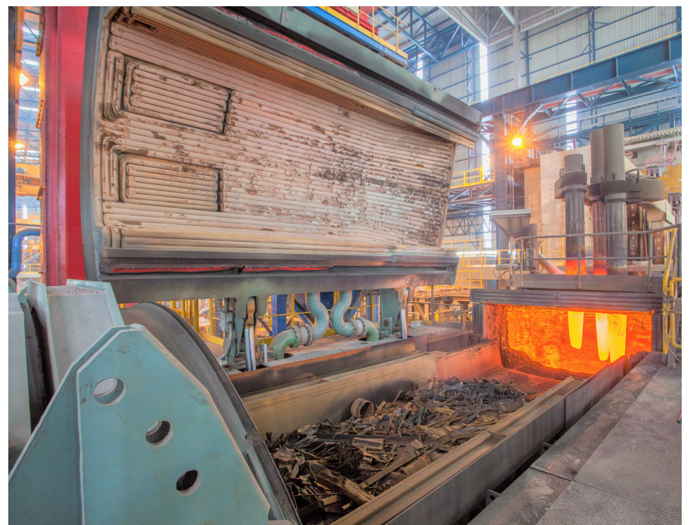
An operational electric arc furnace, similar to the one that will be built in Port Talbot
