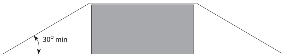
Diagram illustrating an over-the-top restraint with shallow lashing angle.
