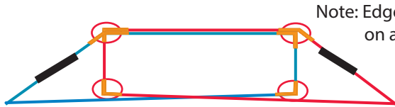
Side by side stacks or parallel stacks: opposing loops wrap around all material in all stacks.
