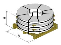
✓ Total height (H) must be less than pallet width (W).
