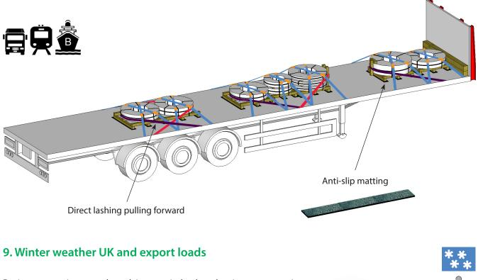
During severe winter weather advisory periods when the air temperature is below 0°C and there is a risk of frost, ice or snow anti slip-matting must be positioned between pallets and trailer deck.
