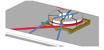
Pallet can be utilized to prevent direct lashing from sliding down.
