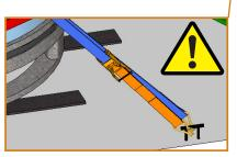
**Note:** If looped straps are required through the spring lashings it is acceptable to put both legs of the looped strap to the same lashing point. This system has been designed not to over-stress the lashing point.
