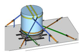
Spring lashings can also be supplied with two 2 to 3 m tails attached. These just require ratchet tensioners to be applied.
