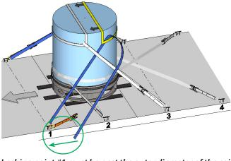
Lashing point #1 must be past the outer diameter of the coil.
