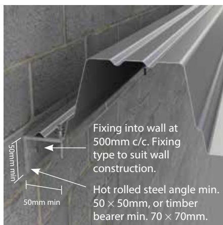
Deck verge detail. Wall abutment
