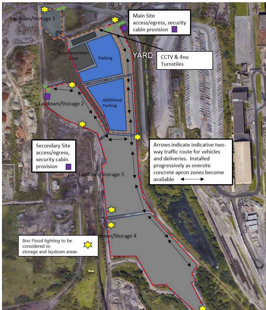
Image 2.10. Proposed construction compound arrangement.
