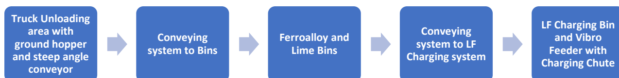
Image 2.3. Block flow diagram of the material handling system for ladle furnaces.
