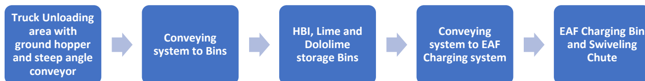
Image 2.2. Block flow diagram of the material handling system for electric arc furnace.
